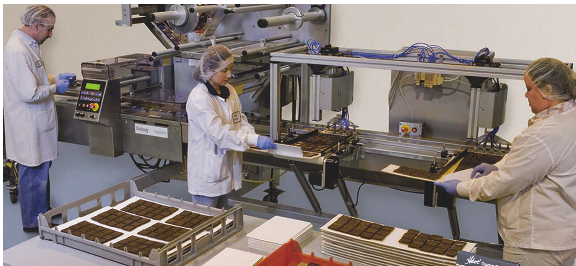
Operators no longer have to place miniBARS one-at-a-time between the spacing lugs on the wrapper infeed chain. The new pick-and-place system is faster and less labor-intensive.
