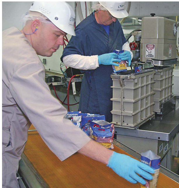
Random samples of Mountain House® lasagna are removed from the conveyor, where statistical process control (SPC) is performed (left). The Windows®-based SPC station gives packaging operators feedback so that adjustments can be made to the filling operation.
