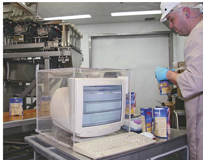
Random samples of Mountain House® lasagna are removed from the conveyor, where statistical process control (SPC) is performed (left). The Windows®-based SPC station gives packaging operators feedback so that adjustments can be made to the filling operation.
